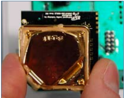
Field replaceable gold-plated CO2 NDIR
