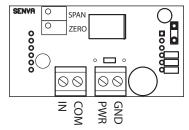
PWRPower supply input positive (+)GNDPower supply ground (-)
