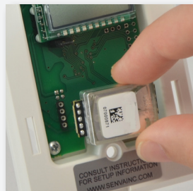
Field replaceable CO2 NDIR element
