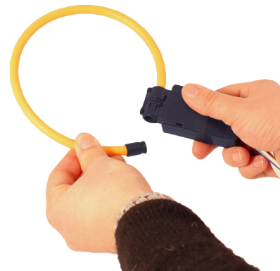
Flexible split-core CVT™ sensors are easy to install and more accurate than traditional CTs
