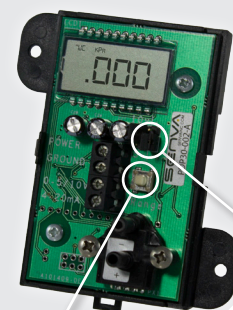
Push button Selectable ranges for high resolution
