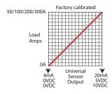
The RoFlexTM provides a universal output signal proportional to monitored current
