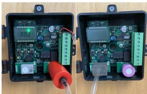
*Gas shrouds secure over respective sensing elements for calibration*
