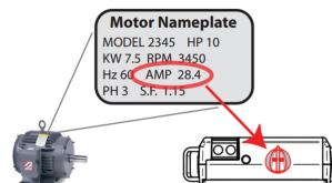
Just set to motor full load amps for proof of flow. Simple and safe.
