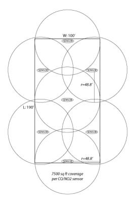
Note: All points inside the structure are within 50' of a Senva TG sensor (for 7500 square foot recommendation). This is a manufacturer recommendation. Consult local and state building codes to ensure coverage is adequate for the monitored space. For sensors covering 5000 square feet, radius should be no more than 39'.
