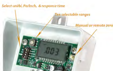
Select measurement & response time. Ten selectable ranges and manual or remote zero.
