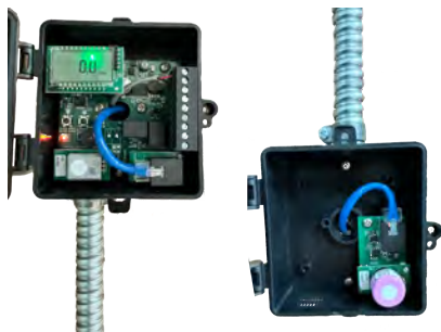
TG-REM kit - mount any 2 gasses at different heights; same as a single device
