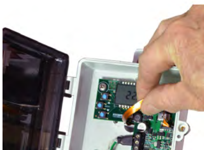
HT ribbon element for harsh environments
