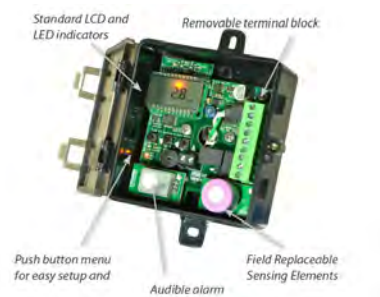
Two sensing elements, buzzer, three color LEDs, and LCD for setup and calibration
