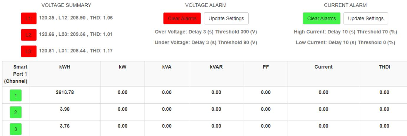
Figure 25. **Detail Data** provides details on each circuit being monitored. The Current Alarm Settings, the same pop-up from the Meter Data tab, can be changed from this page by clicking the Current Alarm "Update Settings" button. The Voltage Alarm Settings can be changed by clicking on the Voltage Alarm "Update Settings" button.
