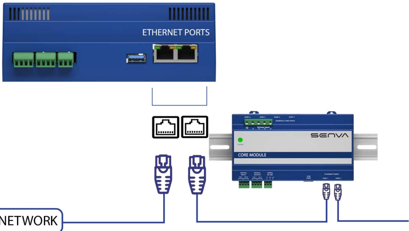
Figure 42. Ethernet port wiring
