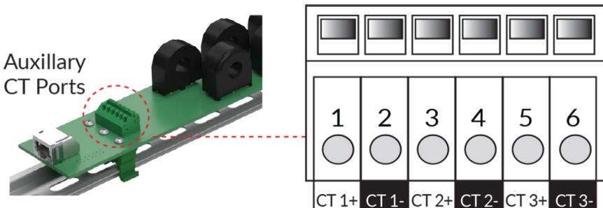
Figure 17. CT strip CT auxiliary ports
