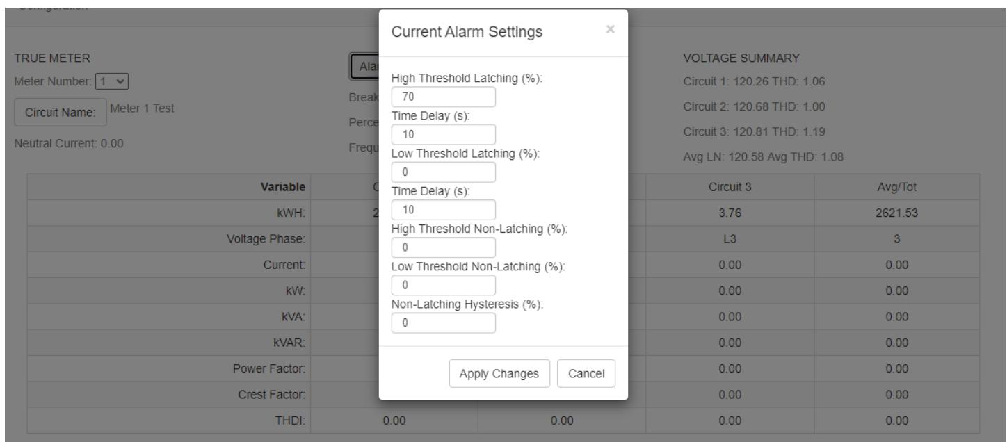
Figure 24. Example pop-up of the Current Alarm Settings.
