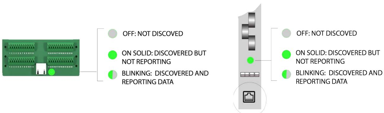
Figure 11. Confirming communication and operation of Interface Card
