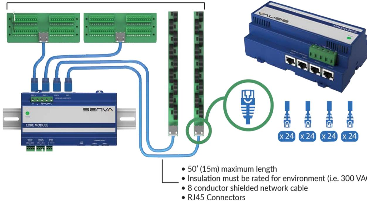
Figure 6. Interface Card Wiring to Core Module
