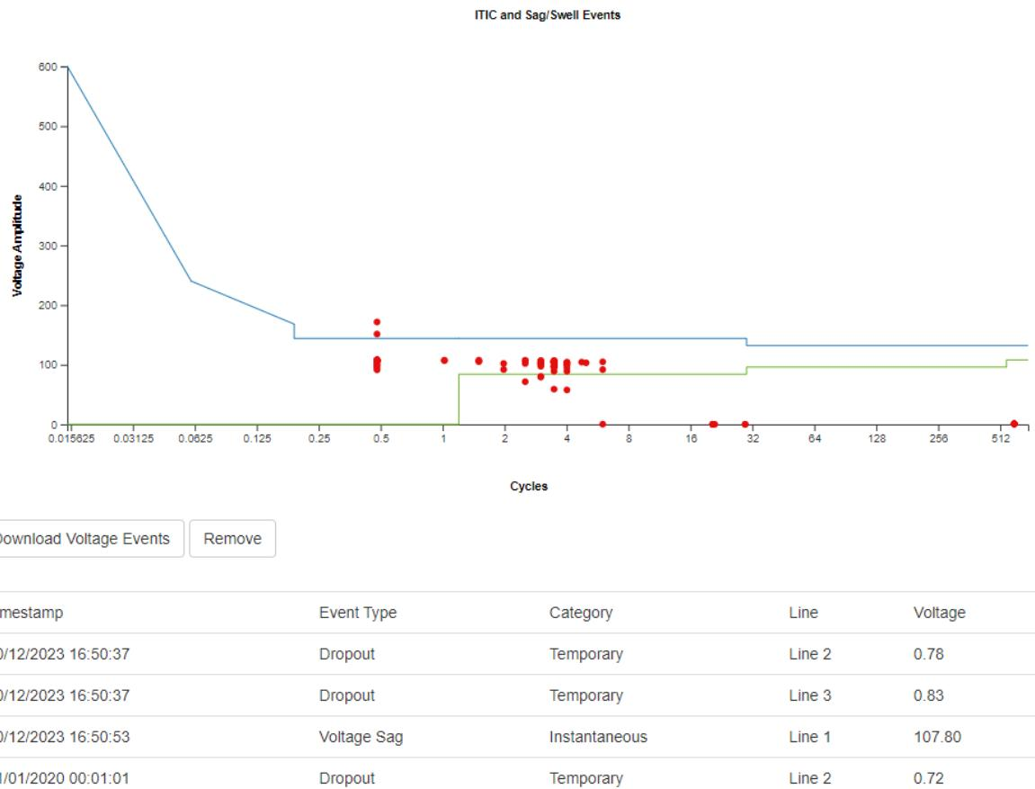
Figure 30. **Voltage Events** shows various events (Dropout, Voltage Sag, etc). This page allows for the removal of the events and the option to download the events to a CSV. The CSV is saved on the computer via the web page and not to the USB stick.
