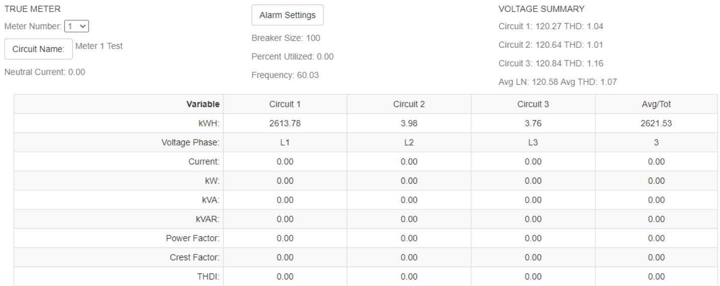
Figure 23. **Meter Data** provides an overview of main input power. True Meters and Virtual Meters can be selected from the Meter Number drop down. Any circuit name can be changed with the 'Circuit Name' button. The Current Alarm Settings can be changed by clicking the 'Alarm Settings' button.
