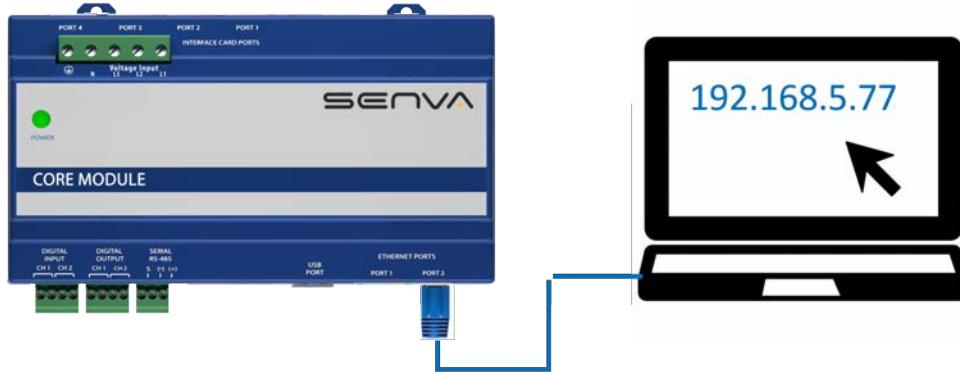
The onboard web console may be used for changing settings and giving a real time view of device readings. This allows it to be used for confirmation of proper operation. Steps for connecting to the Web Console (Splash Page) are below:
