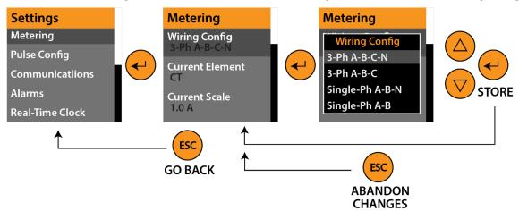
Use the arrows to scroll to select the desired setting, store it by using the enter button and use the escape button to return to the main screen.
