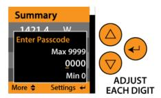
To change any setting, press enter to see the settings menu and navigate to desired parameter and press enter again to choose. For example, to adjust metering parameters, access the settings menu by pressing the 'enter' button once to access settings and once more to access the "Metering" menu and then select "Wiring Config".
