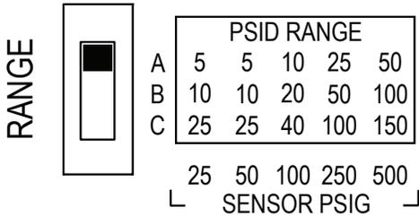
8. Configure product by setting remaining jumpers as shown on diagram. (See 'Configuration Jumpers' section for details on each parameter)
