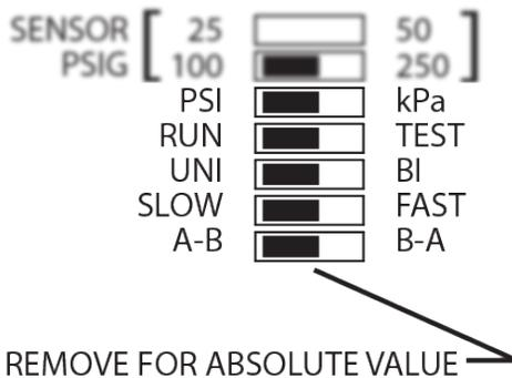
9. Apply power to sensor. TEST MODE jumper may be used to force full-scale output for testing wiring and panel set up. For ZEROING see note (3) below.
