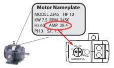
The sensor scale is pre-calibrated for motors operating at a **minimum of 75% FLA**.
